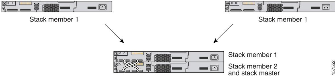
**Figure 5-2** *Adding a Standalone Switch to a Switch Stack*
