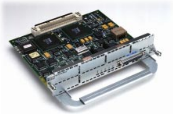
Figura 2 HSSI (High Speed Serial Interface) NM (Network Module)-1HSSI
